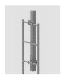
(4) Align the post vertically in the preferred position on the ladder rungs and tighten all the nuts to the specified torque setting.
